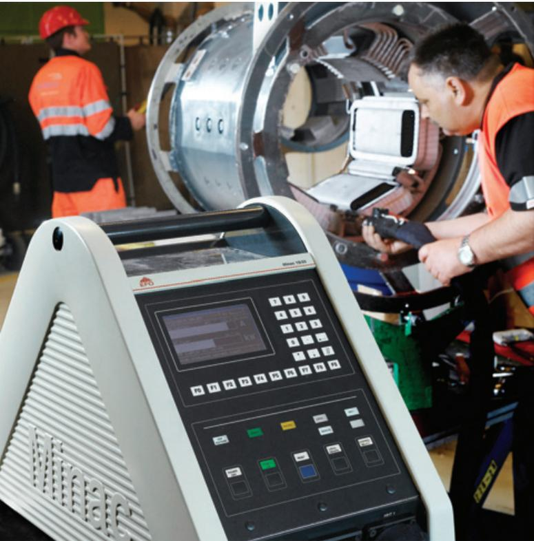
Mobile, flexible and easy-to-use. The Minac brings the benefits of induction heating to tough-to-access workpieces.
