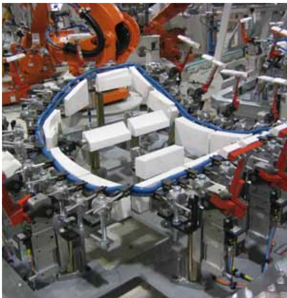
Two of our induction bonding systems. The left photo shows a solution for full-ring bonding. The right photo shows spot-bonding, a method invented by EFD Induction.
