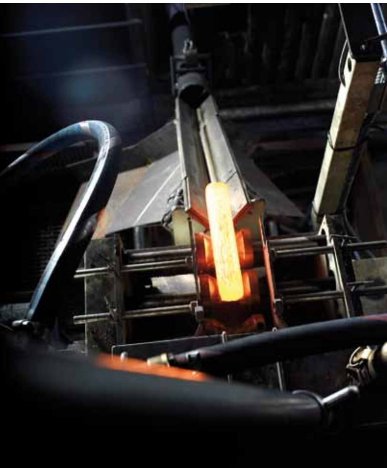
Above, an EFD Induction vertical partial heater. These systems can be fitted with any number of induction coils, and are available in IGBT and thyristor versions.
